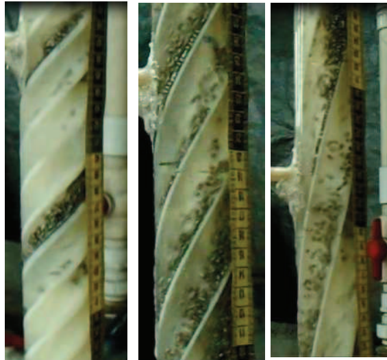
Figure 7. Baffle with 4 starts (from left to right) at 45 °, 60 ° and 75 °.
