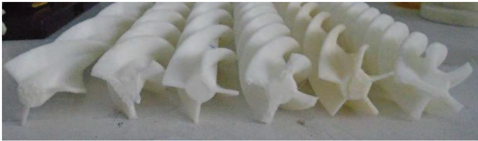
Figure 4. Helical baffles with 3,4 y 5 spirals to 45, 60 y 75 degrees of inclination.
